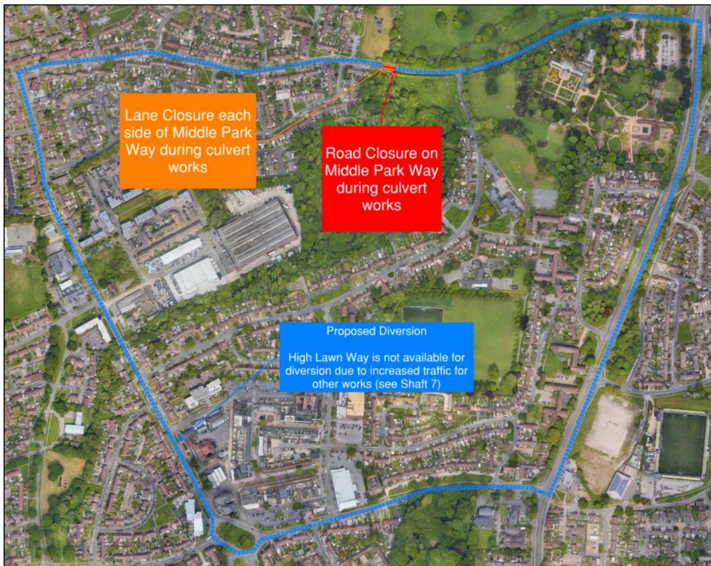
Figure 15-5 – Middle Park Way Road and Lane Closure
