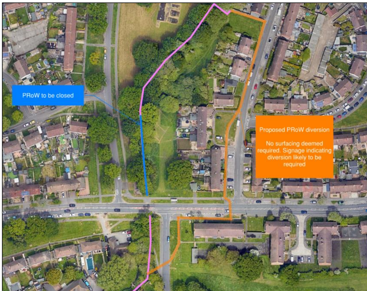
Figure 9-4 – Riders Lane Footpath Diversion
