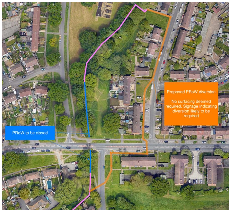
Figure 13-4 – Riders Lane Footpath Diversion
