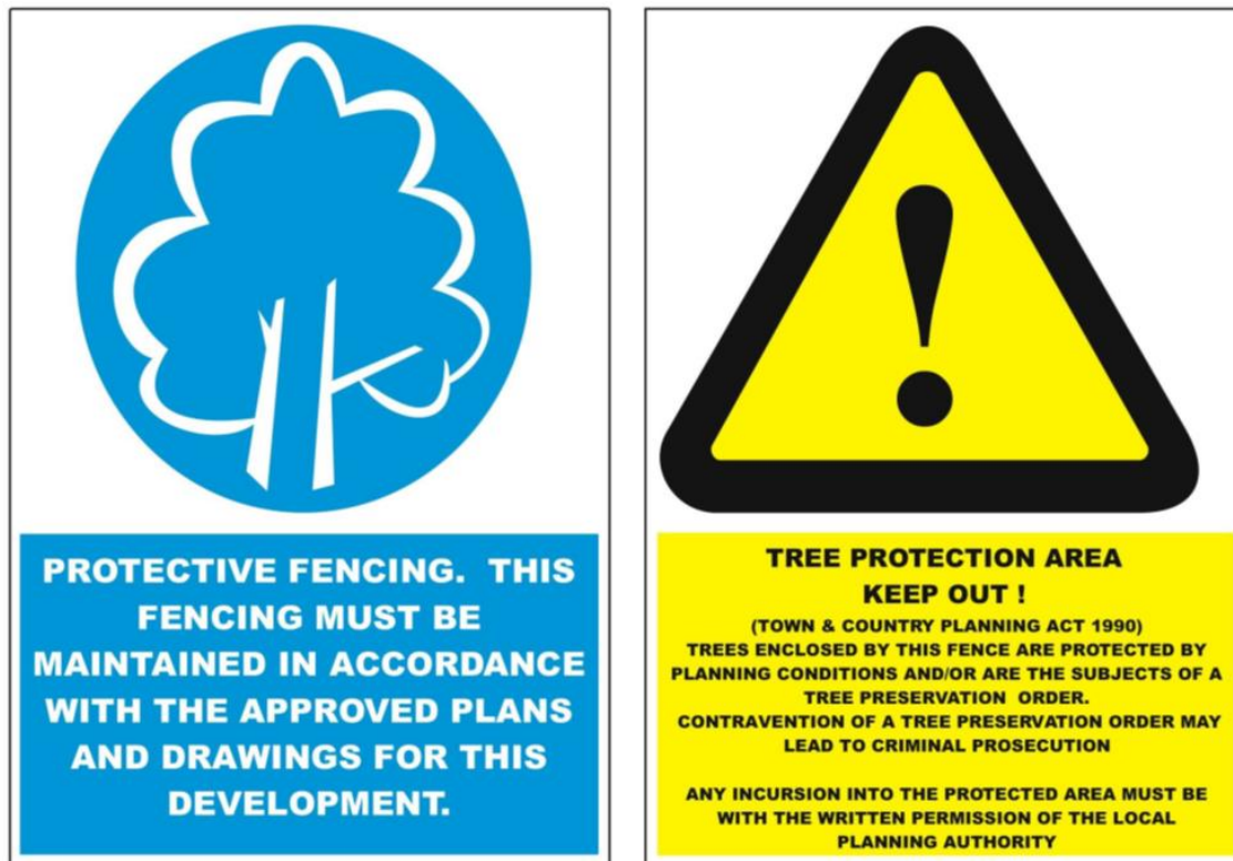
Figure D-3: Example of Protective Fencing Signs
