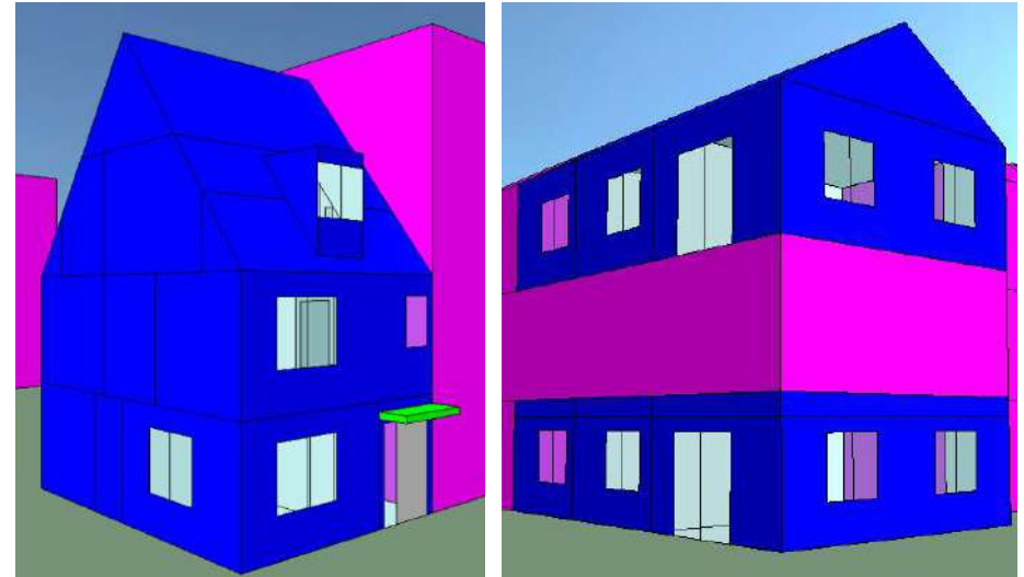
Figure 6: Security issues for window above canopy and GF floor bedrooms in apartments
