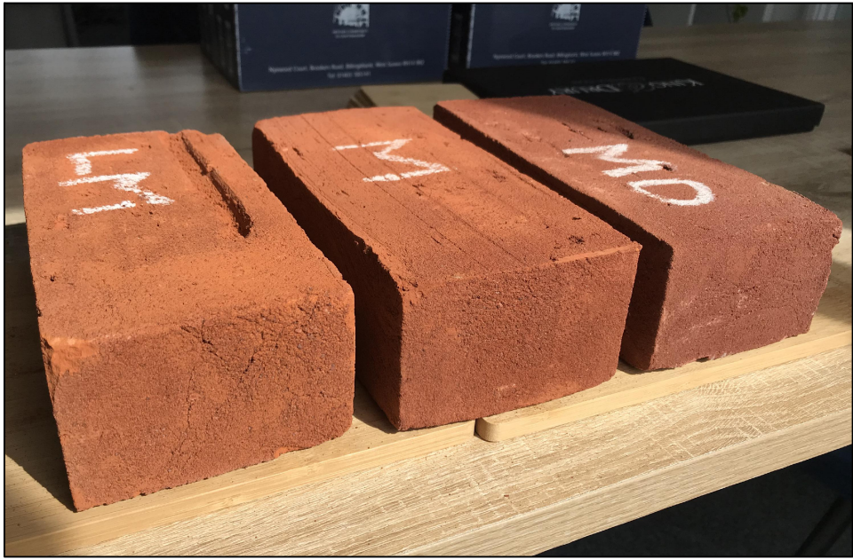
Handmade 'Imperial Red Rubber' facing bricks shown in light (LM), medium (M), and dark (MD). Note specified facing brick to be 'medium' (M).
