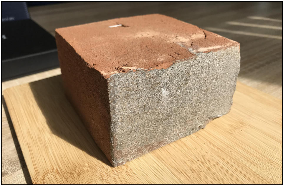
Handmade 'Imperial Red Rubber - Mixed Ash Glazed' header brick.
