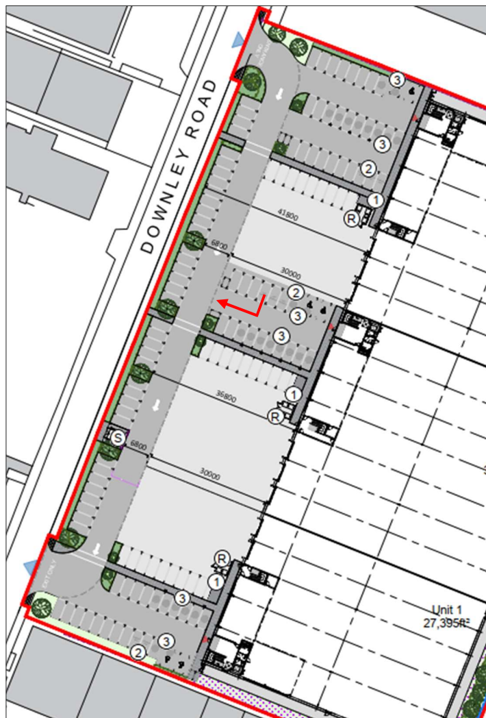
Figure 3-1 Aisle Used to Access Car Parking
