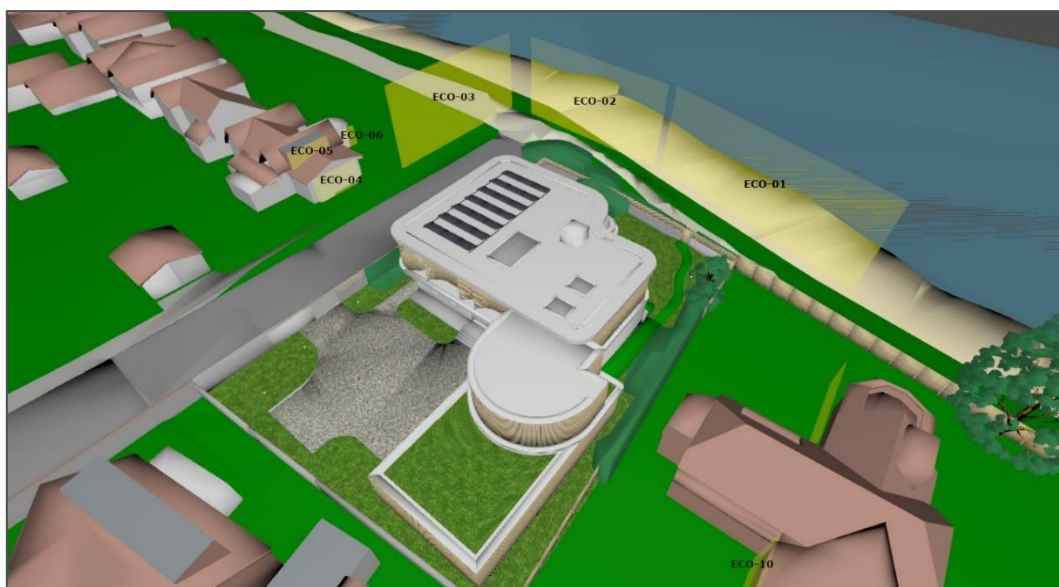
Figure 3: Perspective view of the original model, with the biodiversity vertical calculation Planes. DIALux Software
