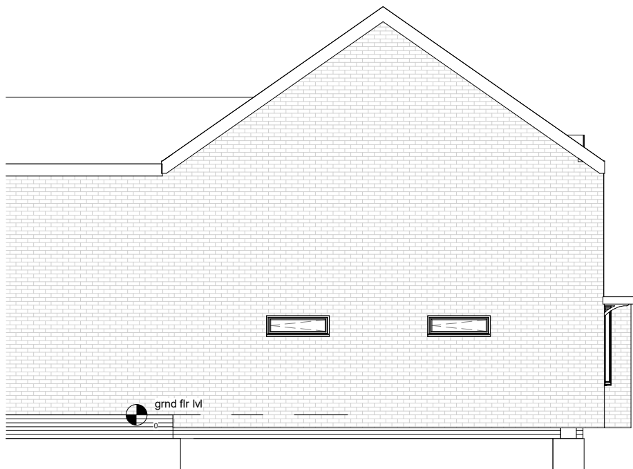
Existing Elevation-Left side
