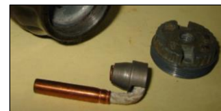
Left: baseplate and detonator removed
