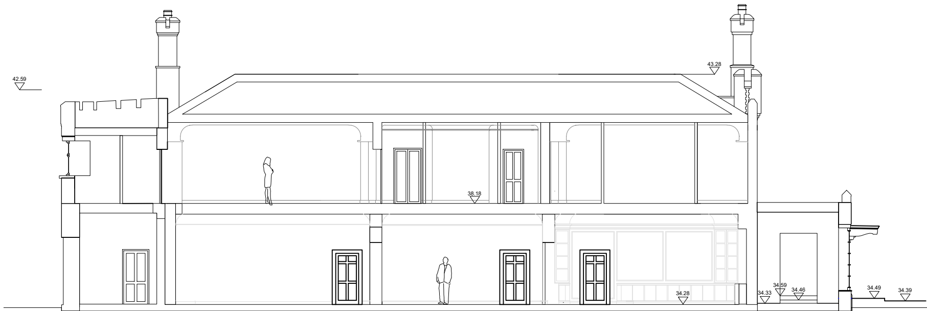
Manor House Cross Section B-B (Proposed) Scale : 1:150 @ A1
