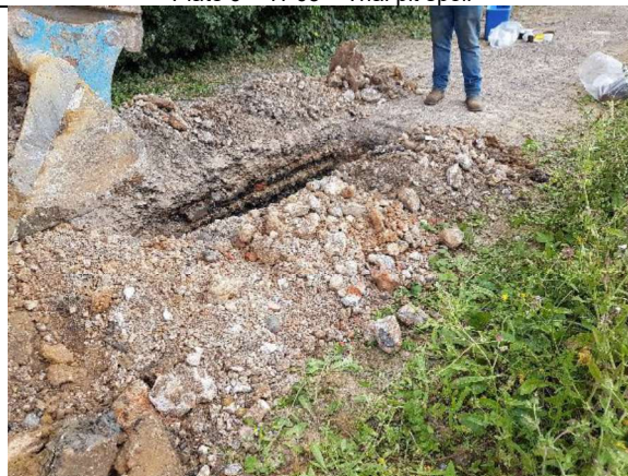
Plate 8 – TP04 – Trial pit spoil
