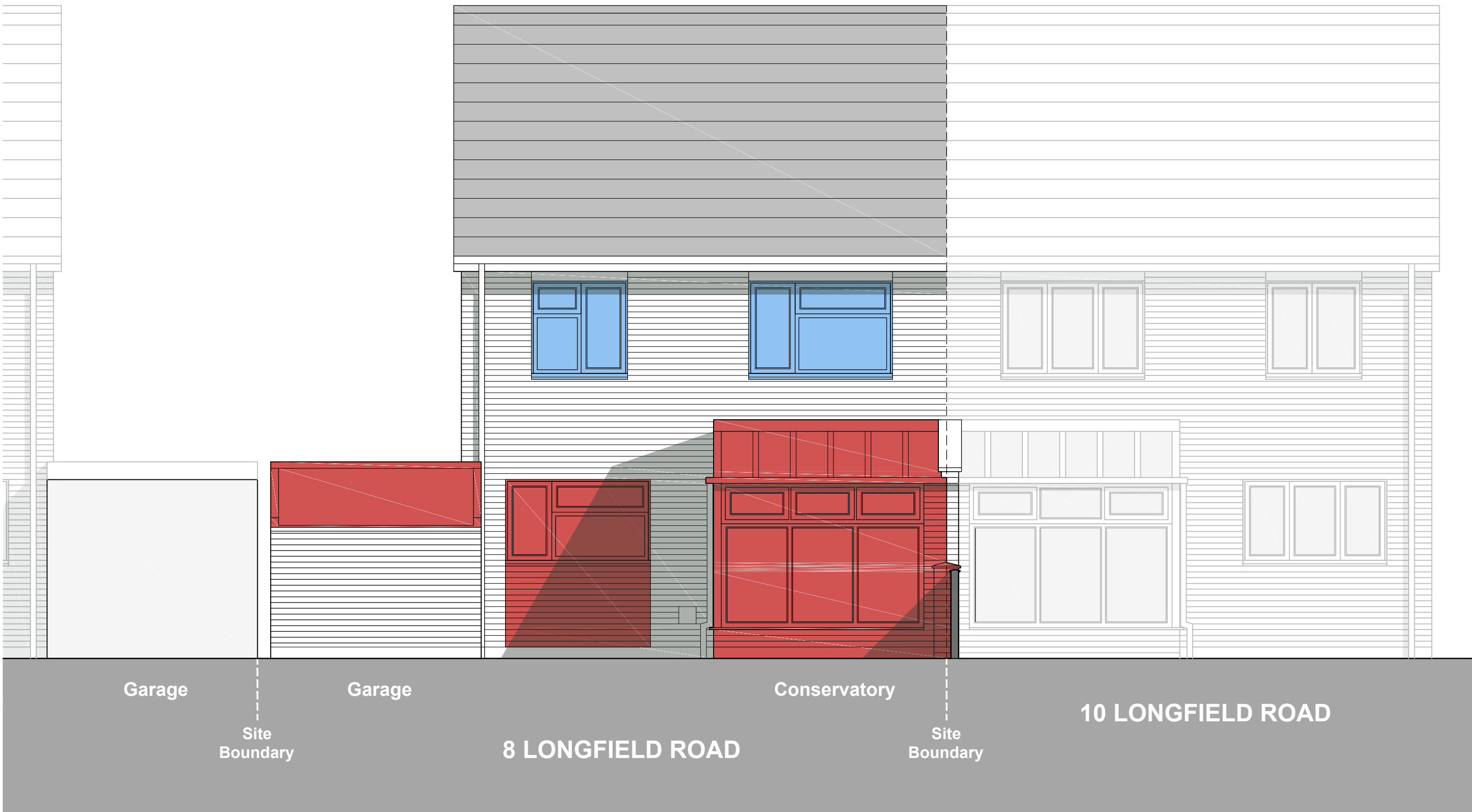
DEMOLITION - WEST ELEVATION
