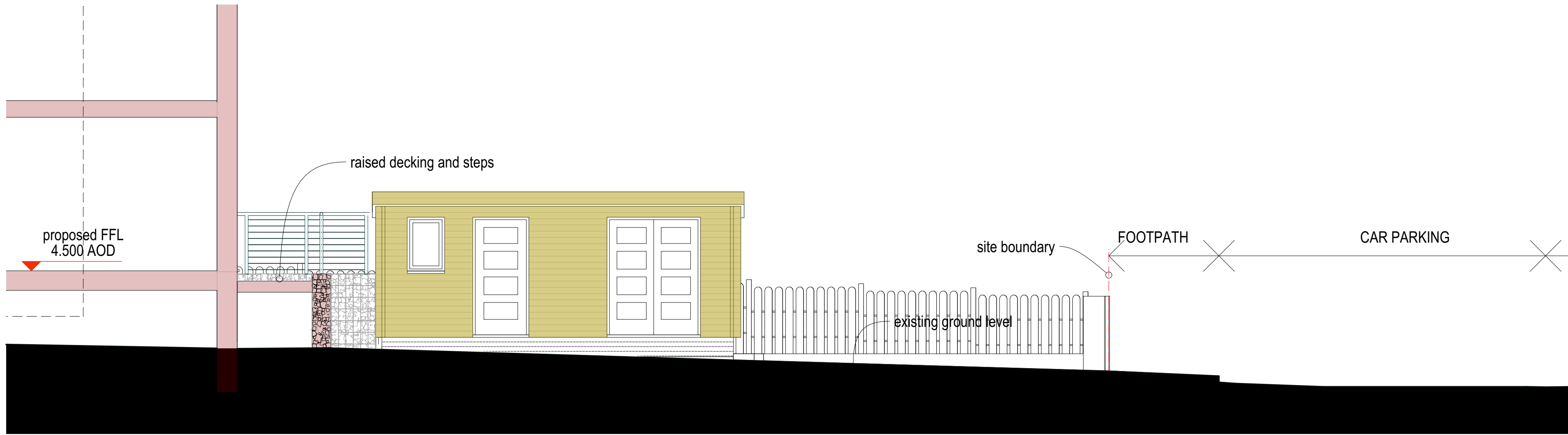
site section and east elevation
