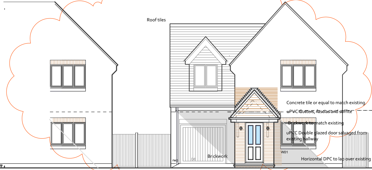
Proposed East Elevation
