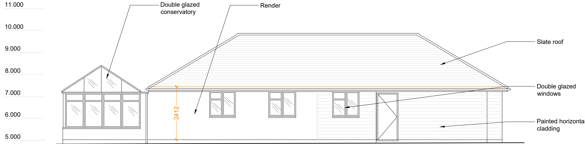
Existing West/Side Elevation
