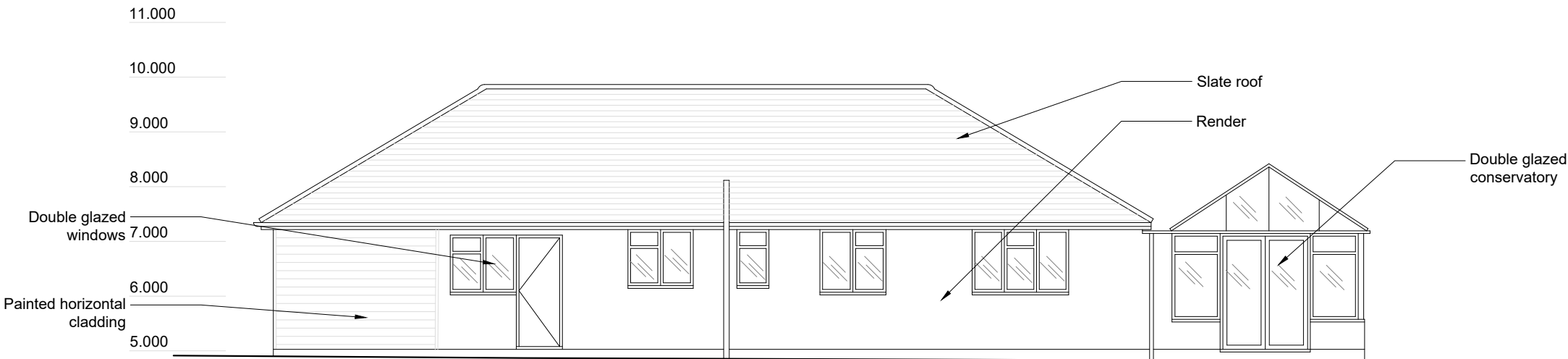
Existing East/Side Elevation
