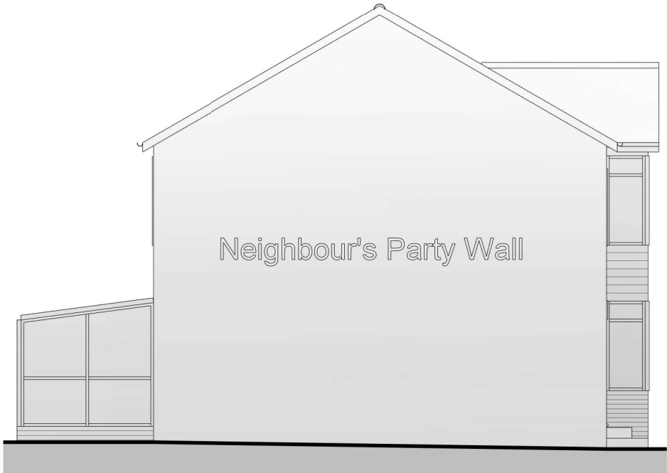
4 Existing Side (S) Elevation 1 : 100
