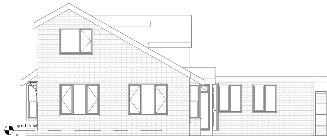
Existing Elevation-Left side
