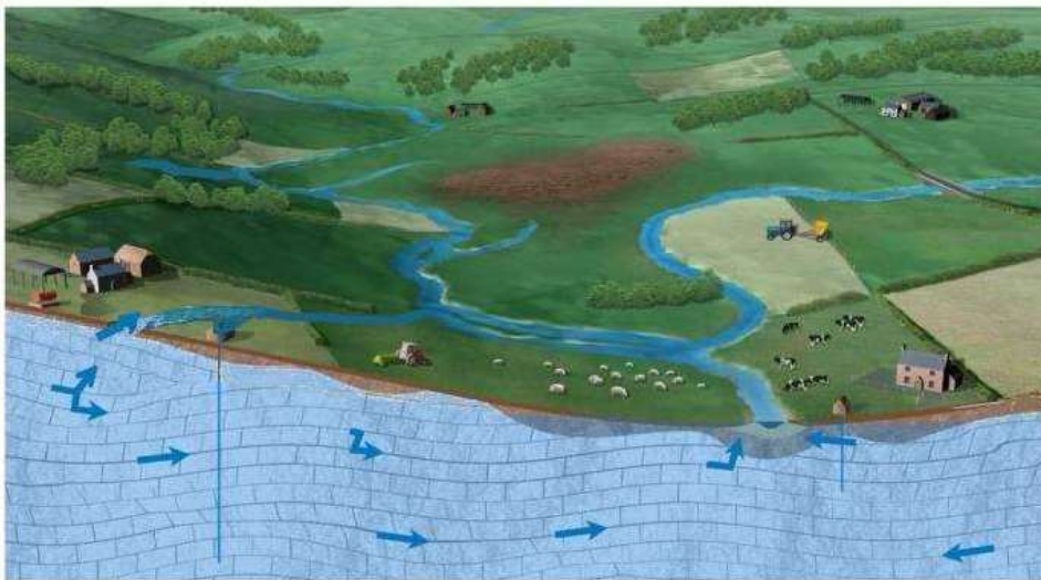
Groundwater emergence (Figure 7.6)
