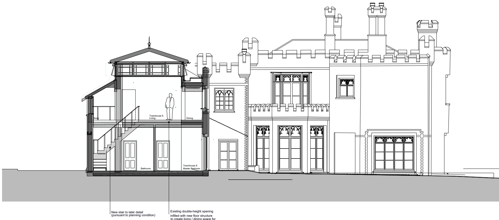
Cross Section C-C [Proposed]
