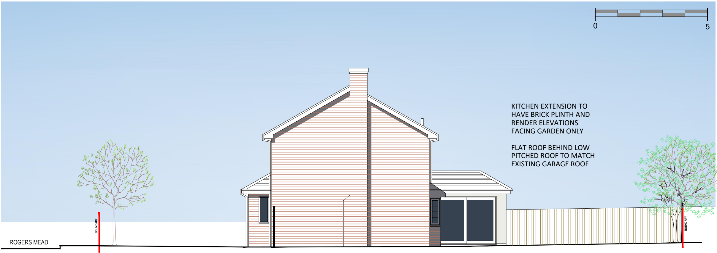
2.0m DATUM SOUTH ELEVATION
