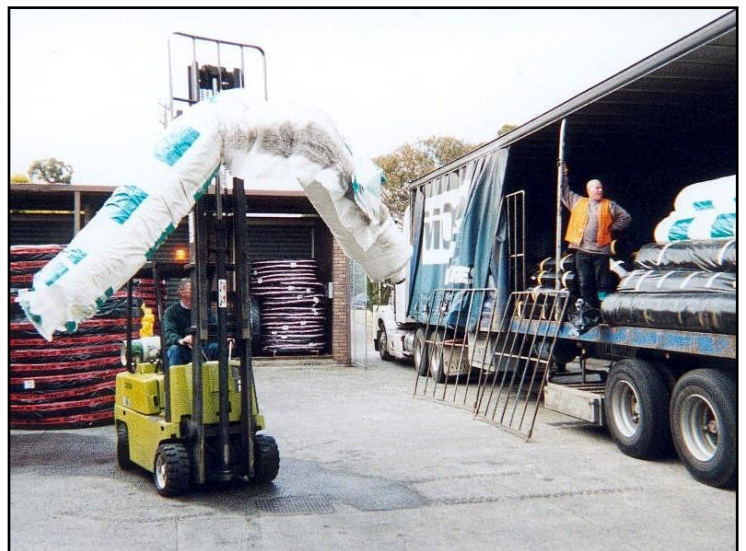
Figure 3 Incorrect method of lifting – must not be used
