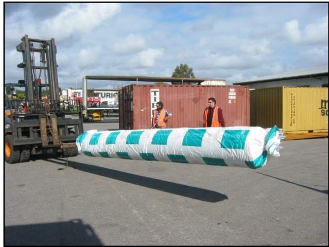
Figure 2 Extracting rolls from container with forklift fitted with a 4m carpet pole
