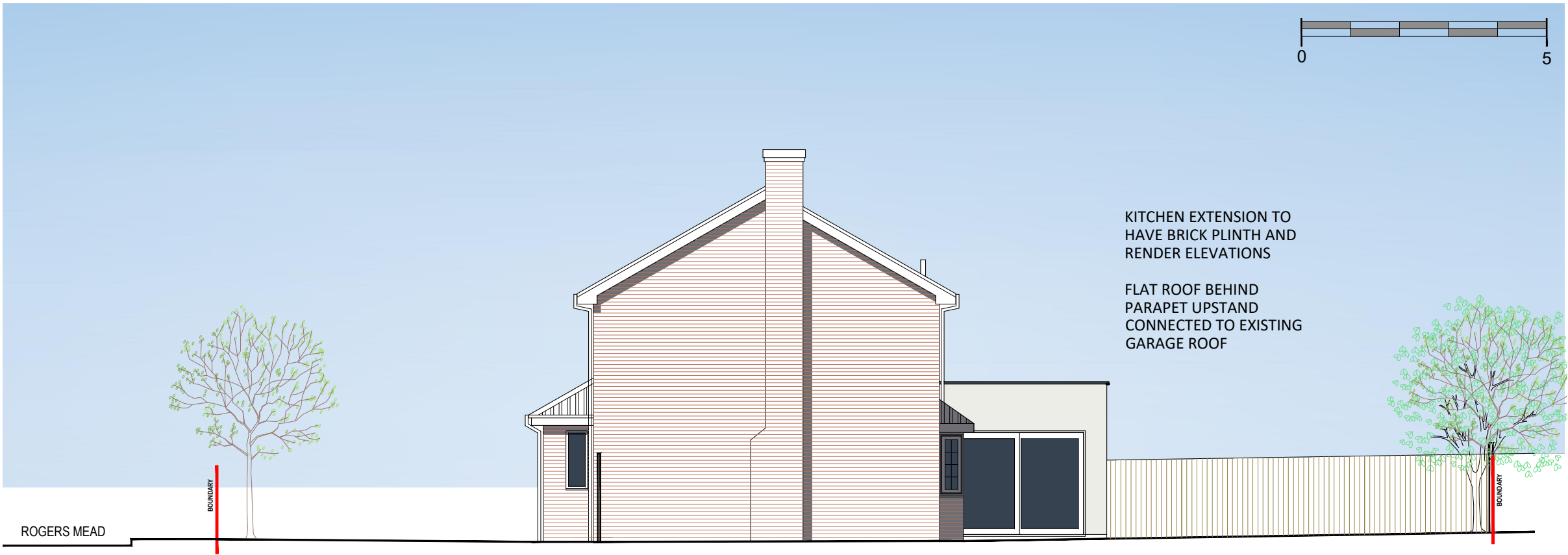
2.0m DATUM SOUTH ELEVATION
