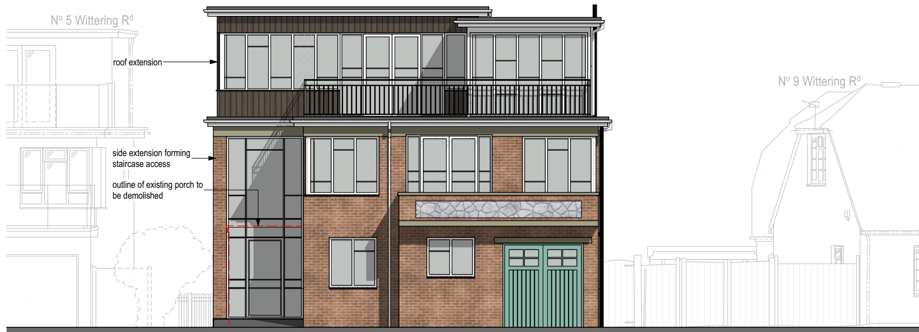
Proposed Front (E) Elevation 1:100
