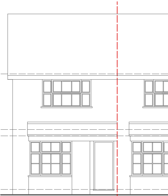
EXISTING EAST ELEVATION 1:100
