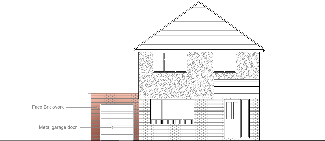
Proposed North Elevation scale A3 1:100
