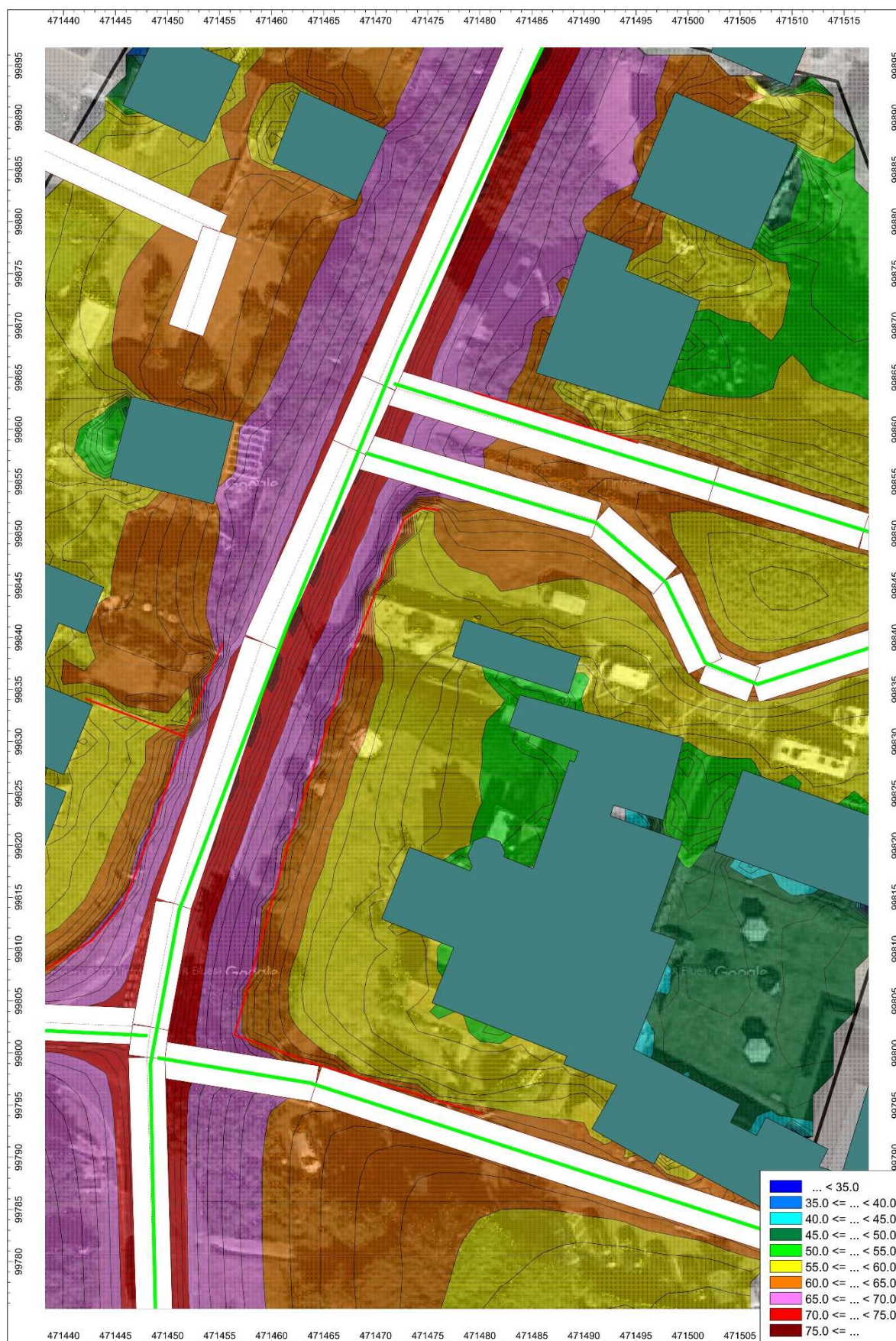
Figure D.1 – Existing site - Predicted dB L_{Aeq,16hr} external ambient noise levels – Daytime (07:00 – 23:00)
