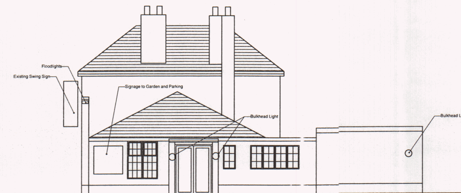
Existing Signage to Side Elevation 1:100
