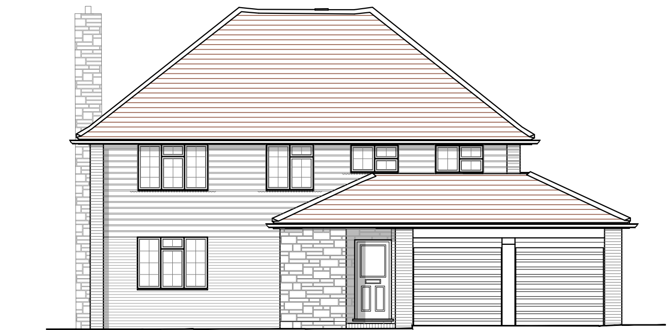
East Elevation [Existing] scale 1_100
