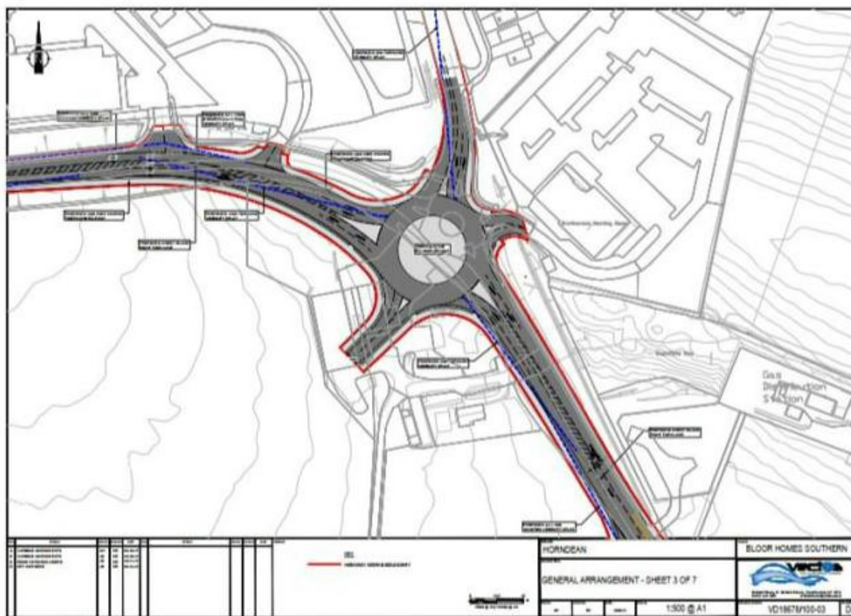
Figure 5-5 - Improvements to the Dell Piece East/B2419 Roundabout
