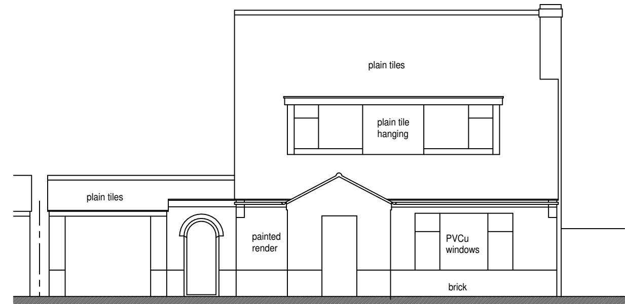
Existing West Elevation
