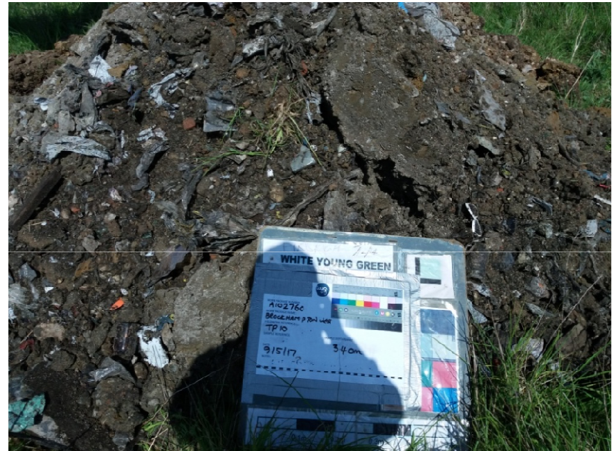
TP10 Pit Spoil – Landfill Material
