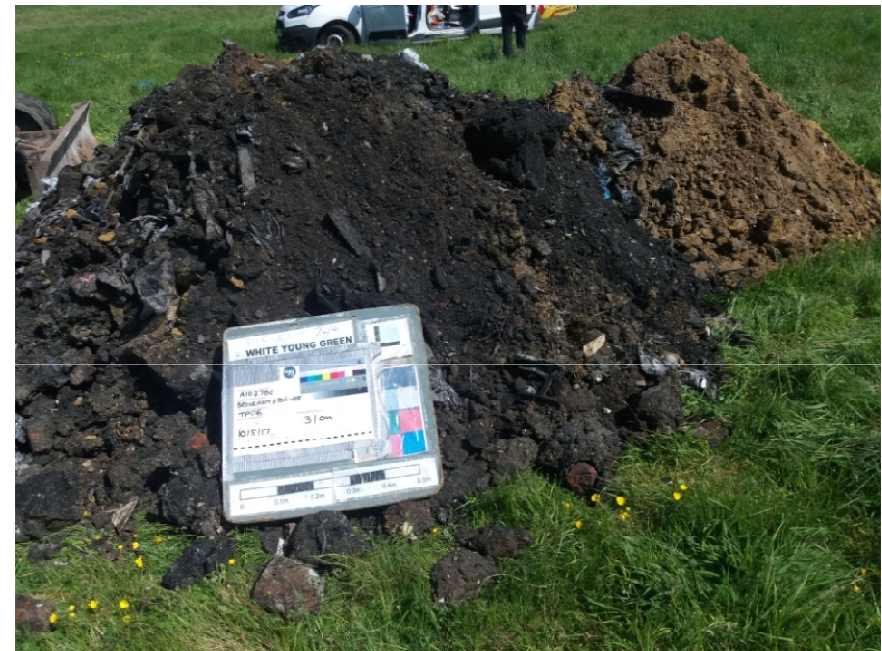
TP06 Pit Spoil – Landfill Material
