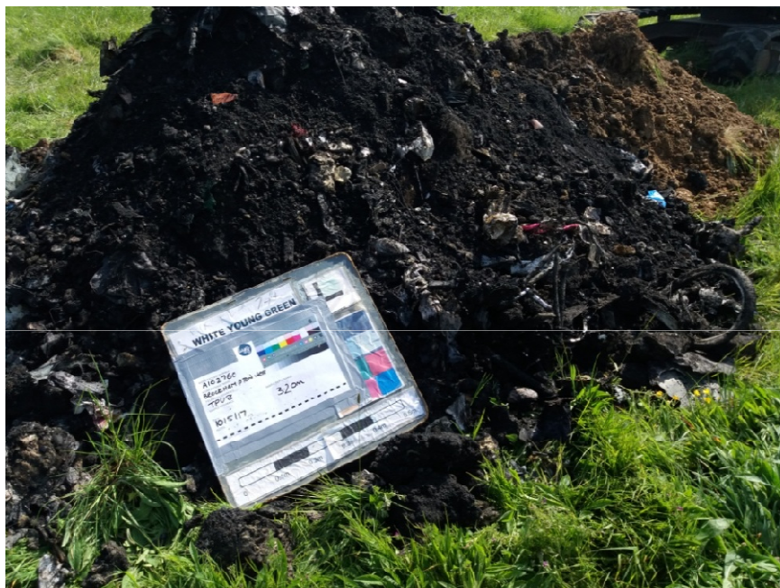
TP08 Pit Spoil – Landfill Material
