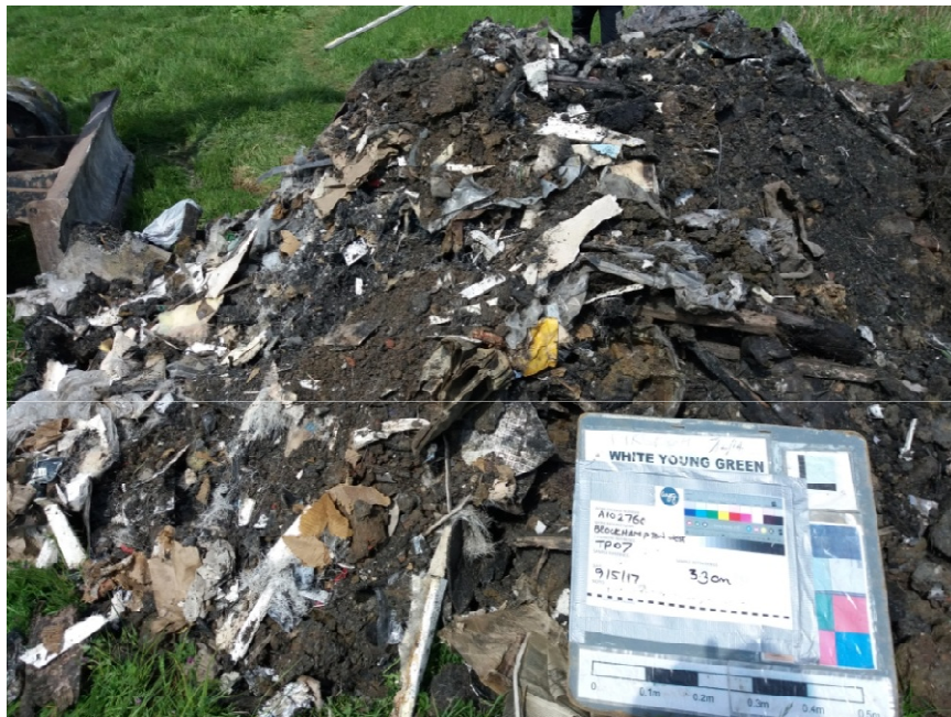
TP07 Pit Spoil - Close up of Landfill Material
