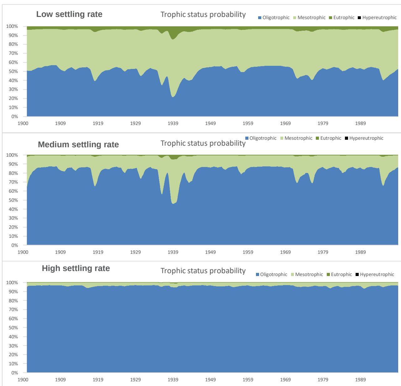
Figure 3.5 Estimates trophic state of the reservoir based on a rolling average of the simulated total phosphorus concentration
