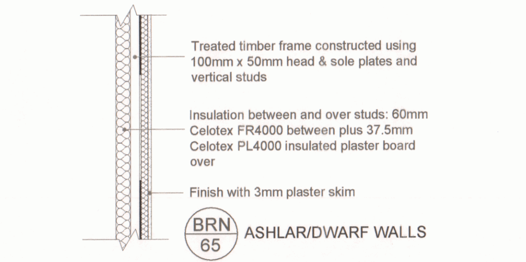
13 PROPOSED ASHLAR WALL SECTION 1:20
