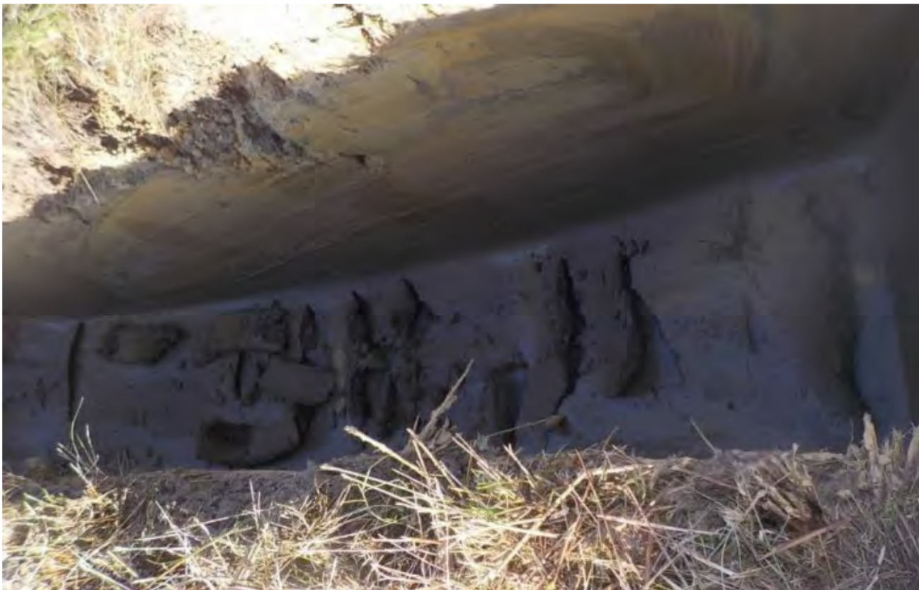
A9031-19 ATK-TP-01 – Examples of Shear Surfaces in clay
