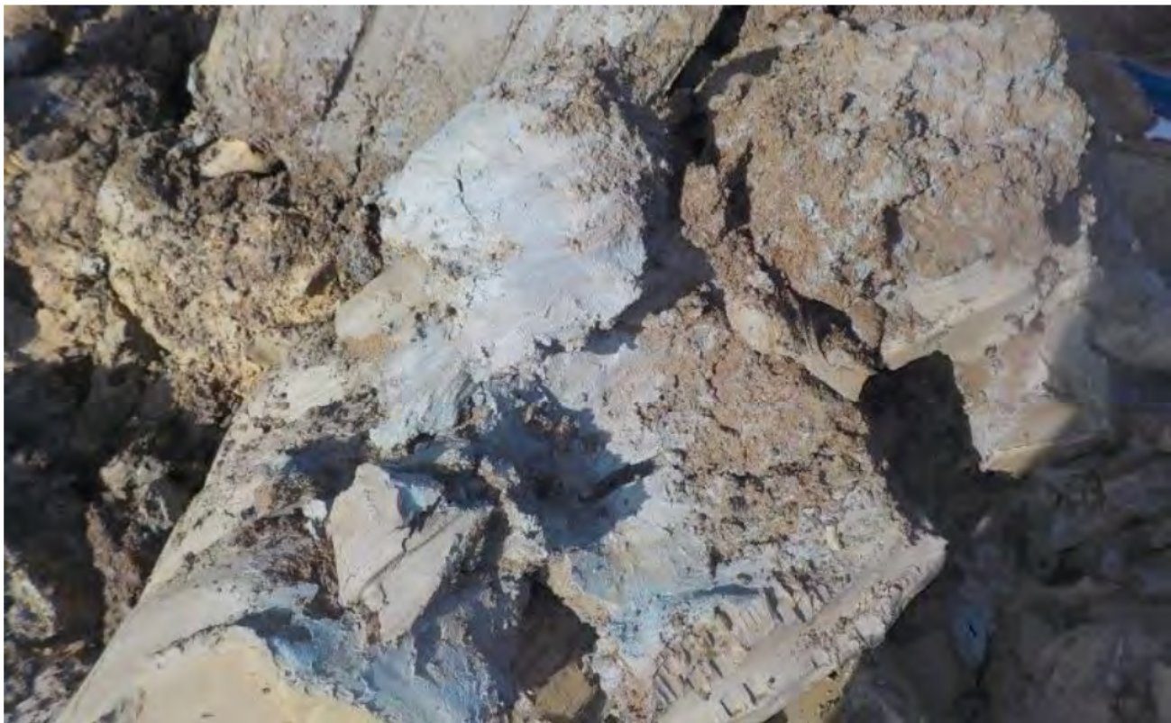
A9031-19 ATK-TP-01 – Example of Shear Surfaces in clay
