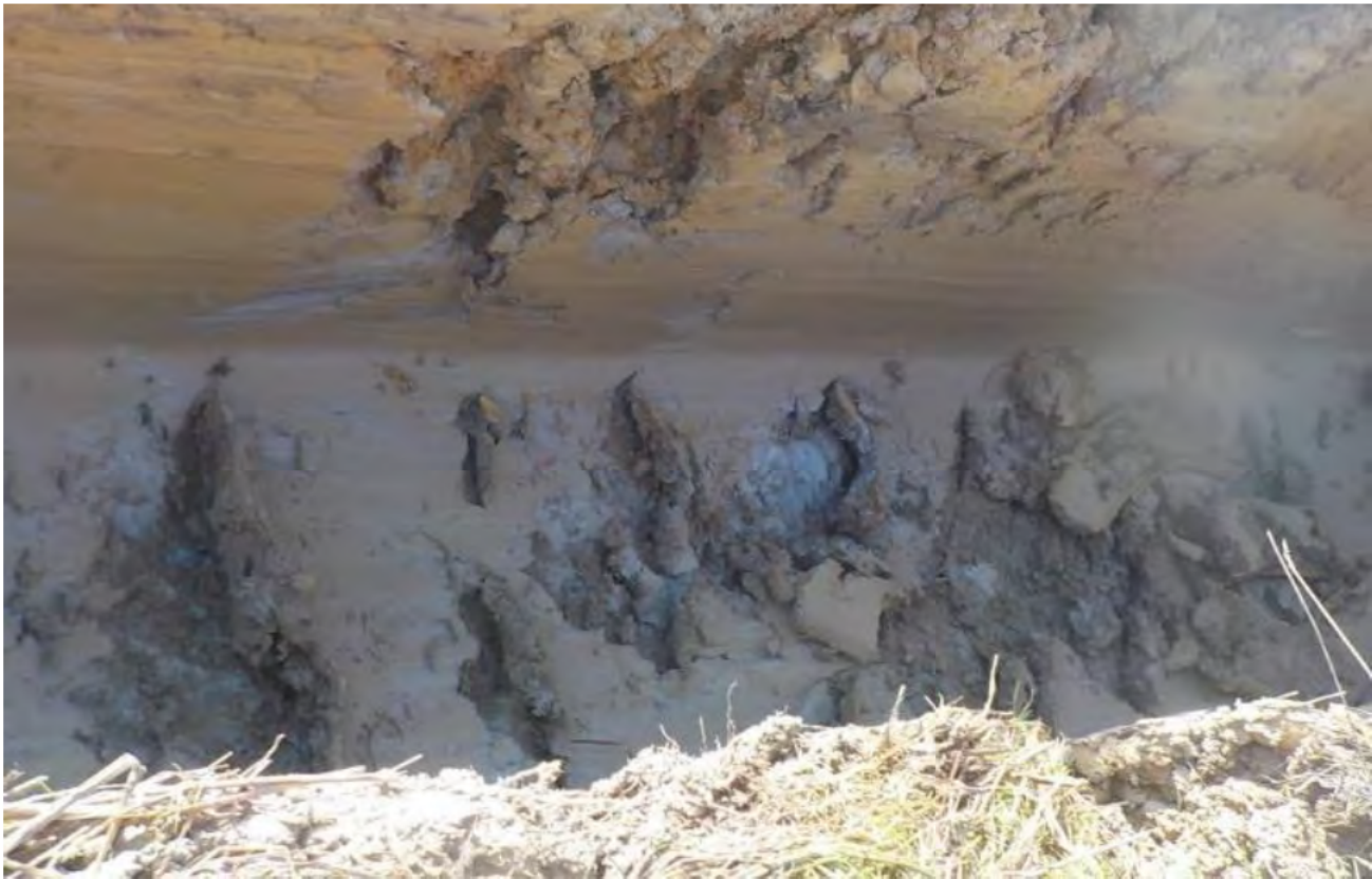
A9031-19 ATK-TP-01 – Examples of Shear Surfaces in clay
