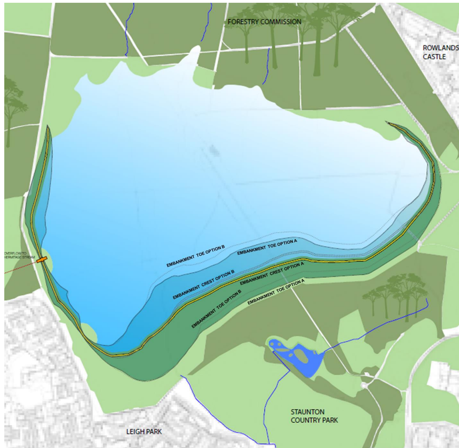
Figure 3.19: Conceptual design of Options A and B showing the projected embankment toes and crests.
