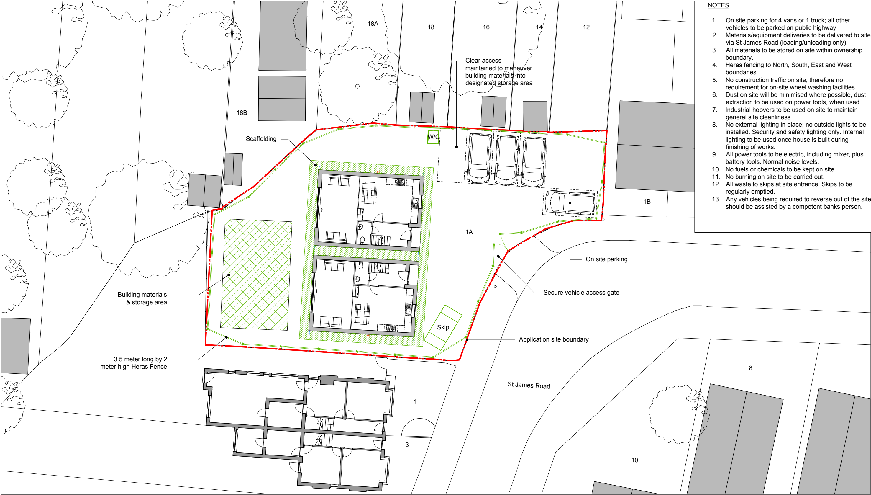
Site Layout Plan - Site set-up during construction
