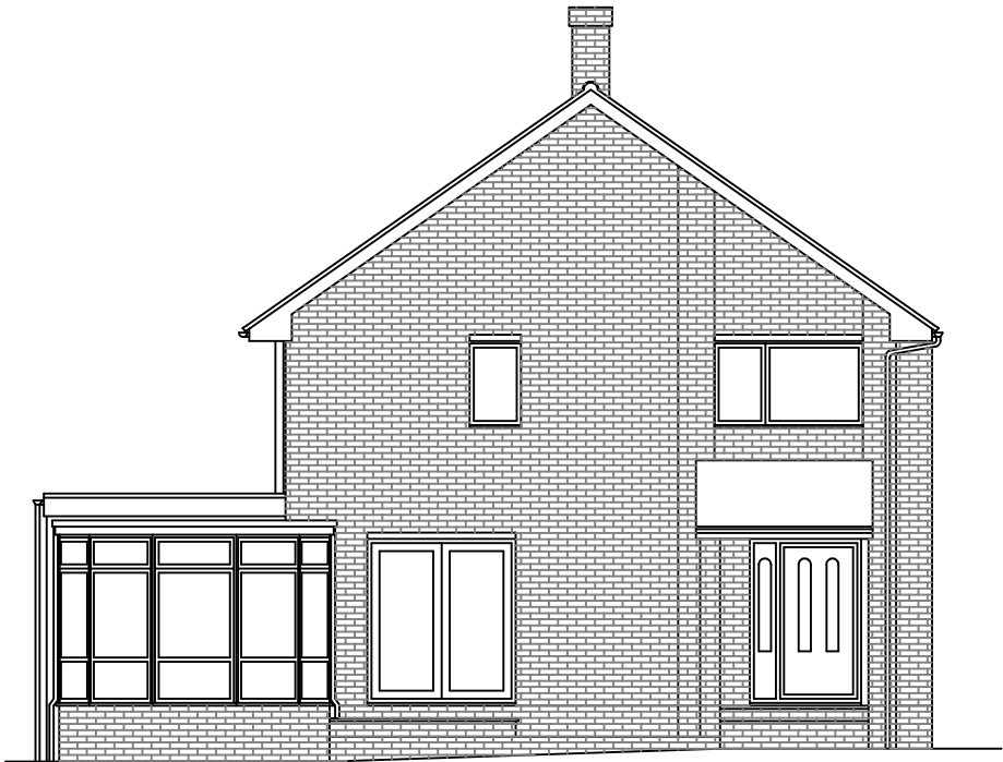
EXISTING SIDE ELEVATION
