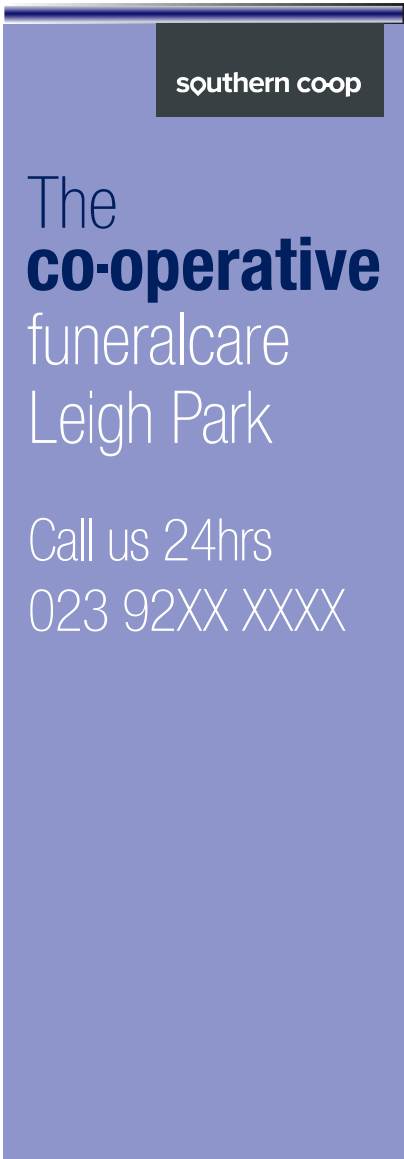
E Trough illuminated 100mm deep totem sign - Aluminium composite pans with cut vinyl graphics applied to face. 3mm built up di-bond tag sign applied to face. SIZE: 1060mm W X 3000mm H
