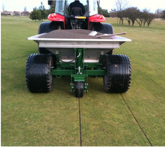
3 Tonne Gravel Band Drainer for large areas
