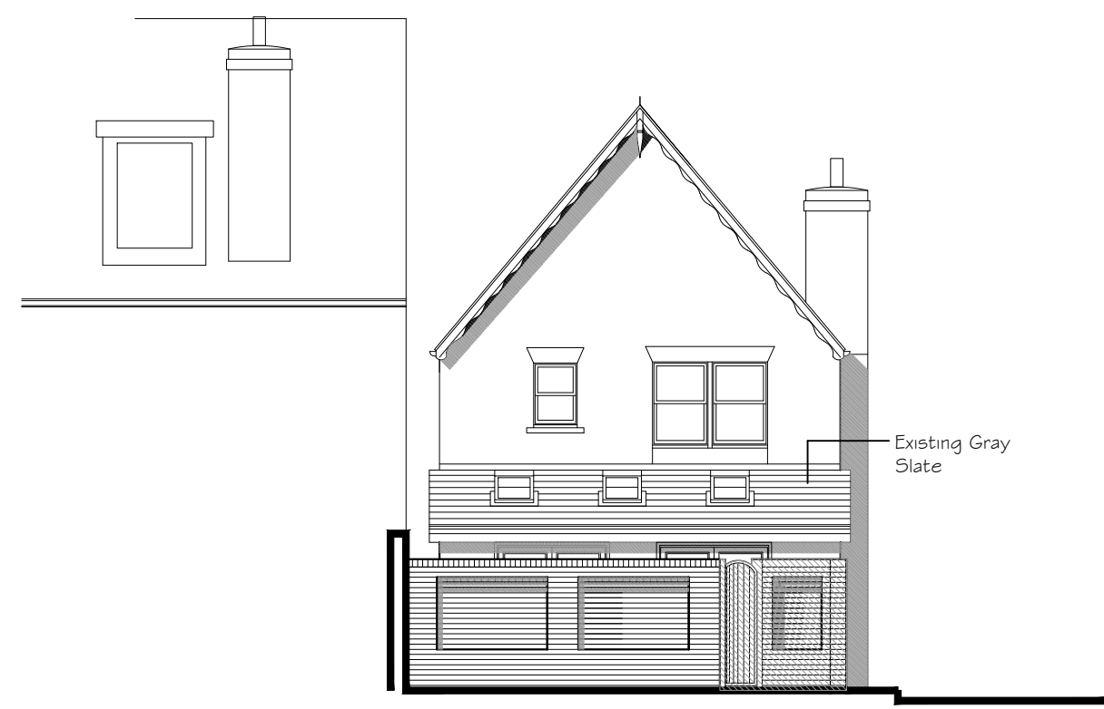
South (behind garden wall) Elevation 1:100
