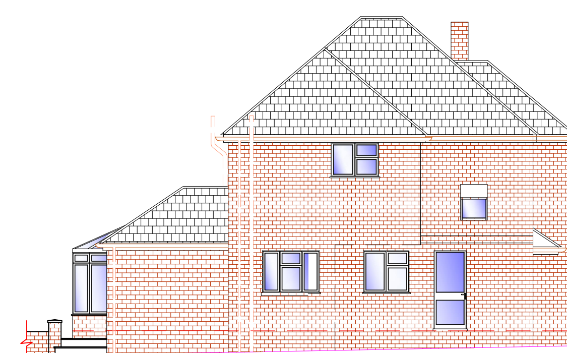
4 EXISTING SIDE ELEVATION 1:100
