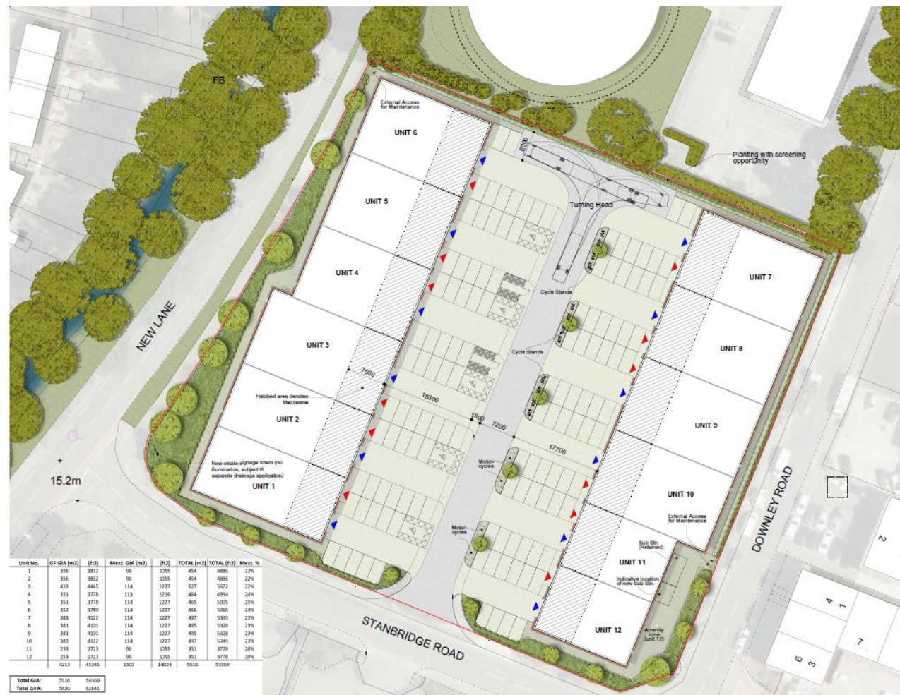
Figure 3 - 18041-HNW-ZZ-ZZ-DR-A-2115 Proposed Site Plan
