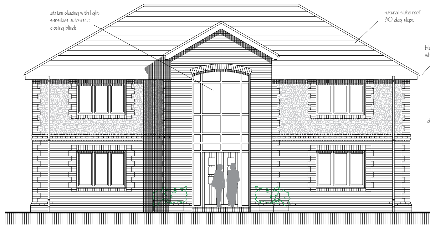
EAST ELEVATION (FRONT)
