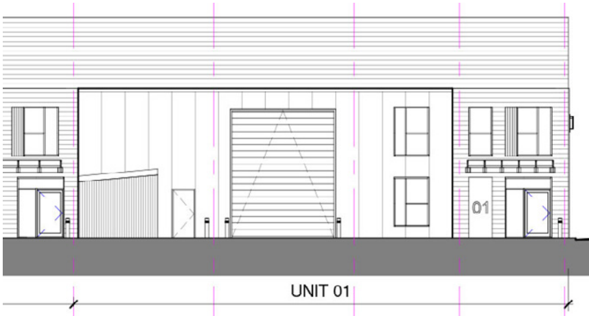
EGRESS DOOR RELOCATION AND BOLLARD INCLUSION
