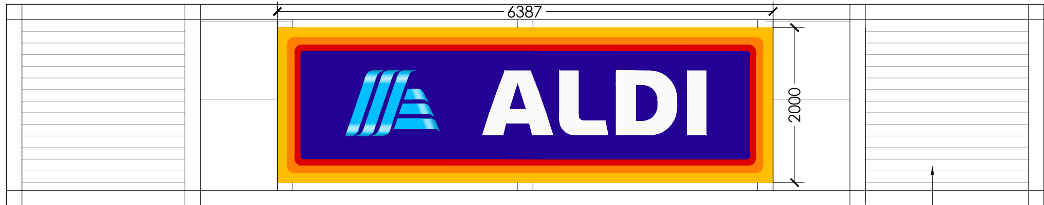
SIGN 01: ALDI CASEMENT SIGN INTERNALLY ILLUMINATED SCALE 1:50
