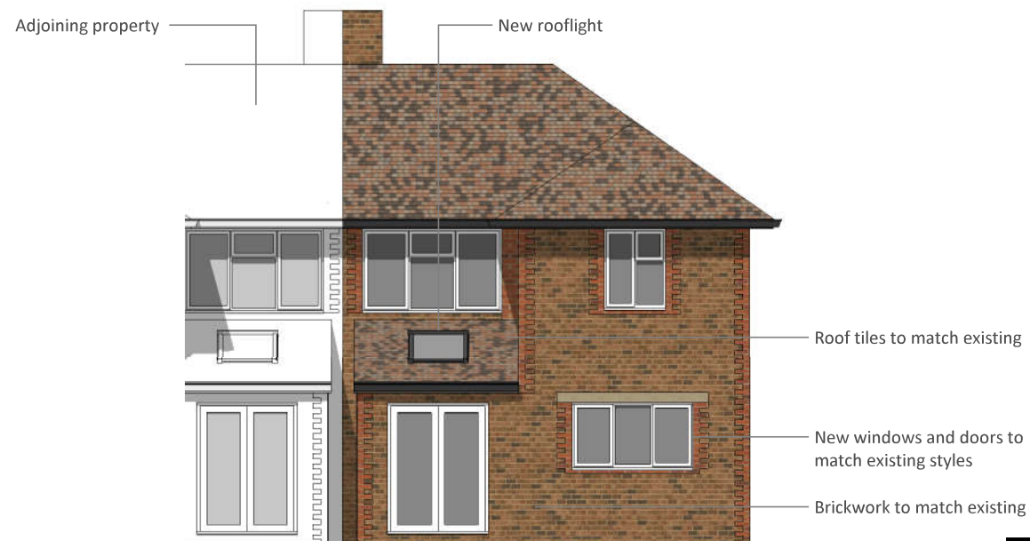
Front Elevation - Facing South
