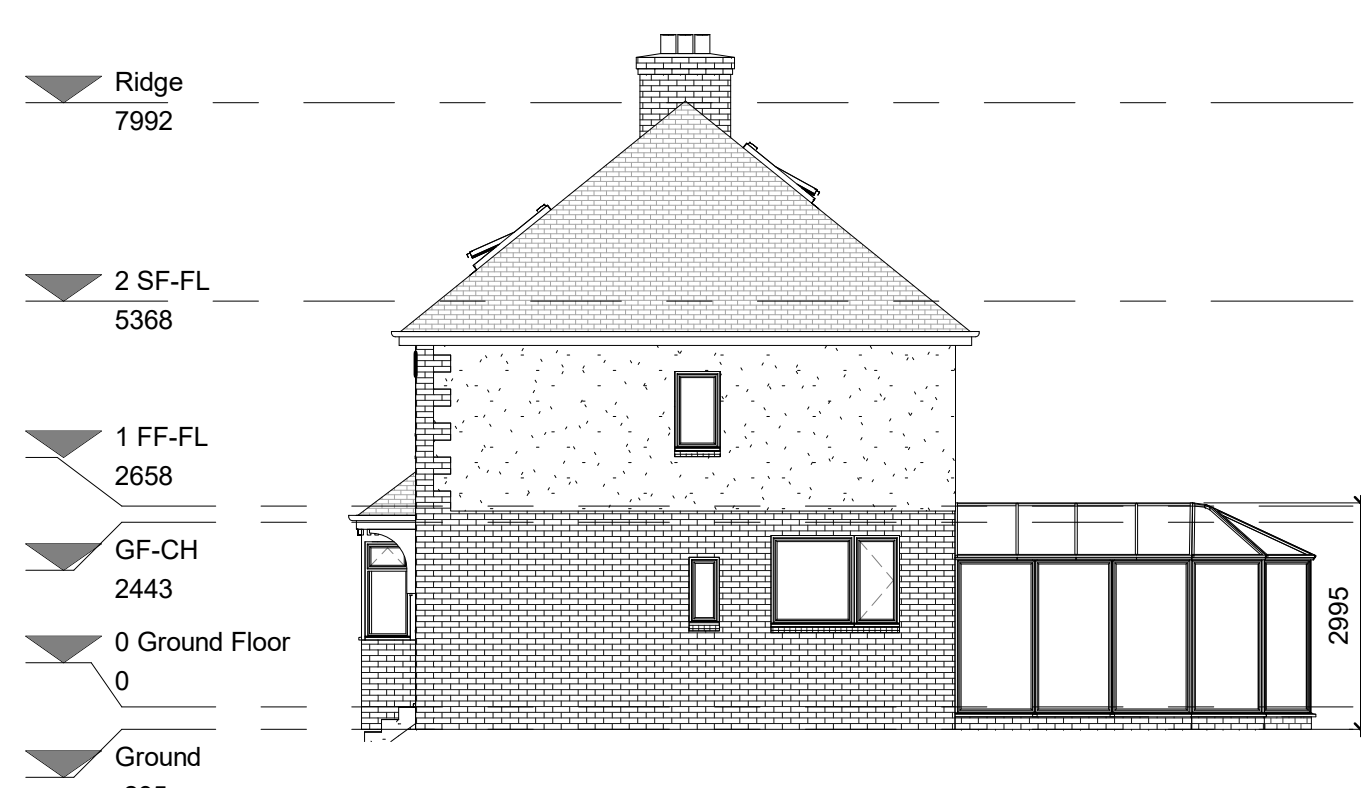
Existing R Side Elevation. 1 : 100
