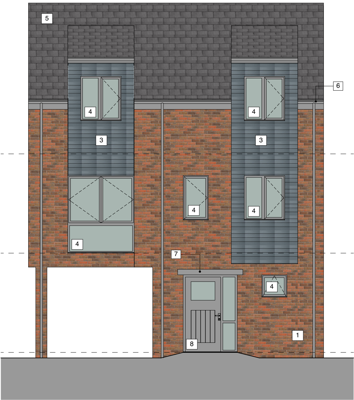
Front Elevation - Facade Treatment B
