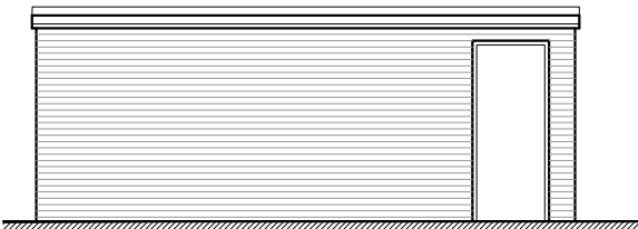
Garage south elevation 1:100
