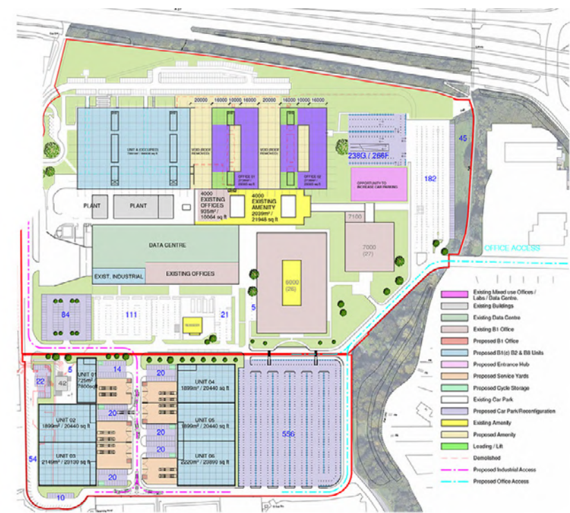
05. Part demolition of B.1000 with the erection of new build offices. New build industrial units south.
